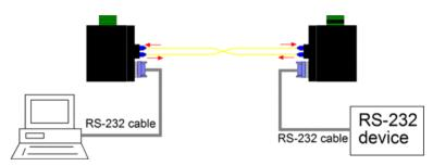
The converter converts all signals of the COM port of the PC to optical signals and sends to the other converter far apart.
