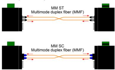
Make sure the RX-to-TX connection rule is followed on the both ends of the fiber cable.
